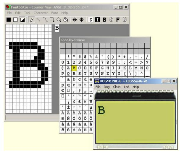
All graphic displays from ELECTRONIC ASSEMBLY EA DOG series do provide a full graphic memory. To display some characters and text, a small bitmap needs to be written into this graphic memory. The FontEditor from ELECTRONIC ASSEMBLY generates those bitmap files. It will be included in  $\mu C$  sourcefiles then.
