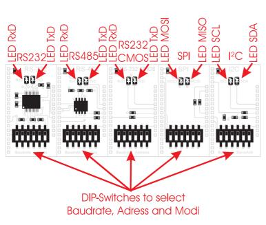
The optional adapter board EA 9777-2PE expands the Evaluation board with important interfaces:
