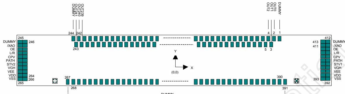
Chip size: 12090 $\mu\text{m}$  x 997.6 $\mu\text{m}$  (scribe line included)
