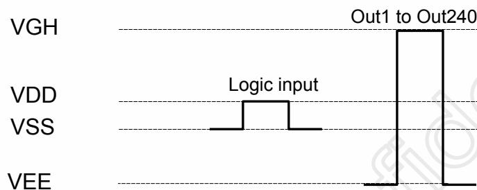
The input signal level of CPV, L/R, OE, STV1, /XAO and STV2 have to swing between VDD and VSS. The signal output level of start pulse (STV1 or STV2) to the next stage cascaded device is VDD for H and VSS for L.
