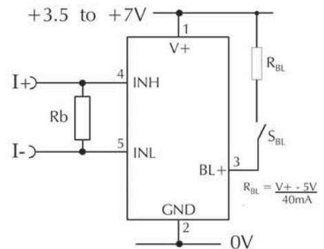
Measuring a current from a circuit which is floating with respect to the DPM's supply, i.e. the current and the meter's power supply are isolated from each other.
