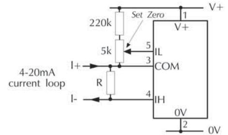
Measuring a 4-20mA loop current. The meter's power supply must be isolated from the 4-20mA current loop.
