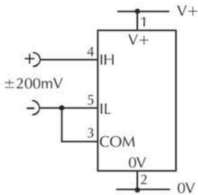
Measuring an input voltage referenced to a floating supply, i.e. the input voltage and the meter's power supply are isolated from each other.
