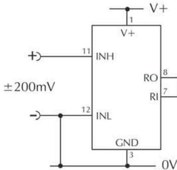
Measuring an input voltage referenced to a floating supply, i.e. the input voltage and the meter's power supply are isolated from each other.
