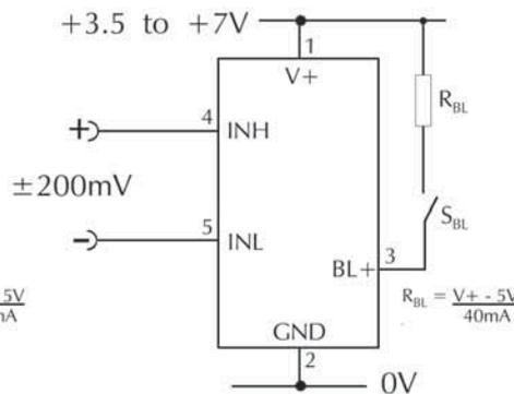
Measuring an input voltage referenced to a floating supply, i.e. the input voltage and the meter's power supply are isolated from each other.
