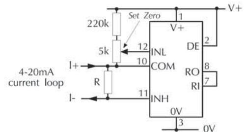
Measuring a 4-20mA loop current. The meter's power supply must be isolated from the 4-20mA current loop.
