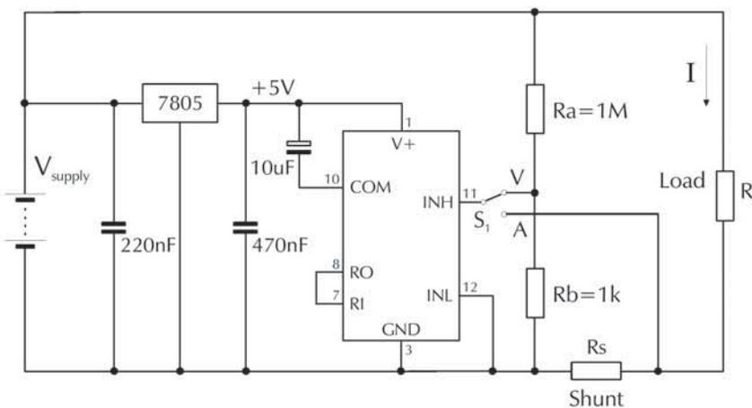
Measuring supply voltage and current to a load. S<sub>1</sub> selects between voltage and current measurement. Ra and Rb shown scaled for 200V<sub>FSR</sub>
