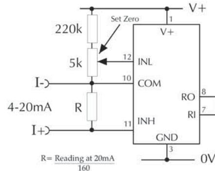
Measuring a 4-20mA loop current. The meter's power supply must be isolated from the 4-20mA current loop.
