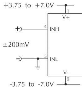
Measuring a single ended input voltage referenced to supply, i.e. the input voltage and the meter's power supply share the same 0V rail.
